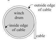
Find the difference in length, to the nearest mm, between the inside and outside edges of a cable 10 mm in diameter that is wrapped around a winch drum of 75 cm diameter.
